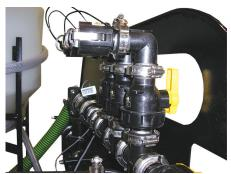
Integrated venturi systems allows the operator to be connected up to three totes at one time. This high capacity venturi will draw product from the bulk containers quickly, getting all the product on board before the sprayer tank is filled with water.
