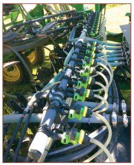
A liquid fertilizer distribution kit that combines "on-the-go" variable rates with precision placement of liquid fertilizer at narrower spacing and various application rates associated with today's seeding methods.
