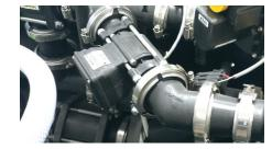
Inductor Pro's can be upgraded to the new Mag meter. The Mag meter provides more accuracy than traditional impeller style meters when being used with higher viscosity water based products.
