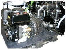
Proven performance - powered by a 13 hp PowerPro electric start motor the 3 in. Hypro pump will deliver up to 440 gpm.
