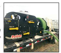
Batch tank with a capacity of 30 USG, allows for the easy mix of powders and liquids. The tanks rinse system, with integrated fresh water quickly cleans jugs removing all contents of the tank.
