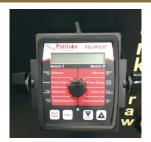
The Flo Pro II monitor, Is capable of monitoring two individual meters. Pre-programed the monitor will activate batch control valves to open, allowing product to be metered. When the desired amount of product has passed through the meter it will automatically close the valve.
