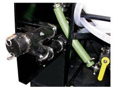
High quality Banjo 3 in. leak proof manifold style fittings will provide years of trouble free service. Raised handles on all valves for easy maneuvering.
