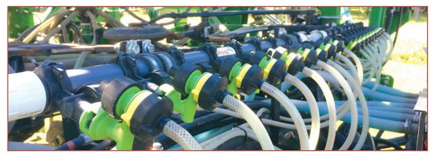
A liquid fertilizer distribution kit that combines "on-the-go" variable rates with precision placement of liquid fertilizer at narrower spacing and various application rates associated with today's seeding methods.
