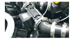
Inductor Pro's can be upgraded to the new Mag meter. The Mag meter provides more accuracy than traditional impeller style meters when being used with higher viscosity water based products.
