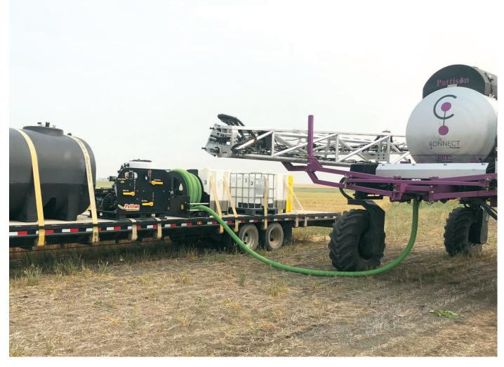
Shown above is the Pattison custom built spray trailer being used to fill the new Connect SP120, Dot ready implement. On board the trailer is the Pattison Inductor Pro II and hose reel.
