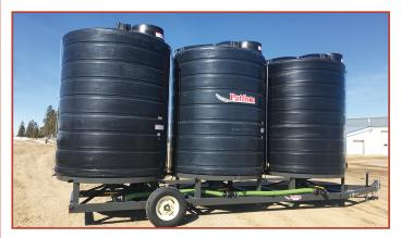
Pattison Field Storage Unit, is available in the triple tank configuration with a total capacity of 9000 usg. The unique hydraulic jack system easily raises and lowers tank platform. The 3" plumbing allows for quick load and unloading with the tanks having a 10 degree cone bottom to ensure a total drain. Only transport the tanks empty.
