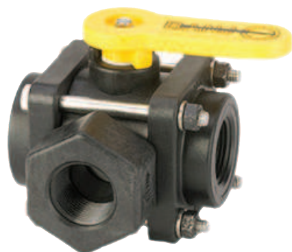
Side Load: Directional flow, right or left. Valve cannot be turned off.
