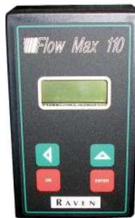
Raven FLOmax 110 combined with the Raven RFM 60P meter displays metered units in US gallons or litres. One Step calibration with accuracy of +/-1%, is compatible with most agricultural products. Will calculate flow rates, batch and total volumes.
