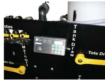
Available as an option is the Flomax 810. The Flomax 810 when integrated with a shutoff valve, allows the operator to pre programme a batch volume. When the correct amount of product is measured out the Flomax 810 will automatically close the intake valve.
