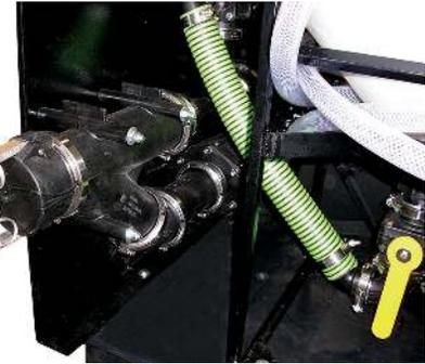
High quality Banjo 3 in. leak proof manifold style fittings will provide years of trouble free service. Raised handles on all valves for easy maneuvering.
