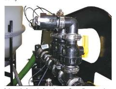
Integrated venturi systems allows the operator to be connected up to three totes at one time. This high capacity venturi will draw product from the bulk containers quickly, getting all the product on board before the sprayer tank is filled with water.
