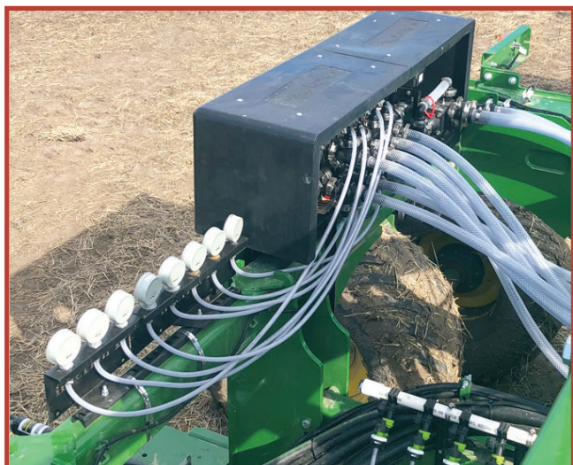
Picture shown: RAXARC auto rate control package with RAXBOOM8 sectional control
