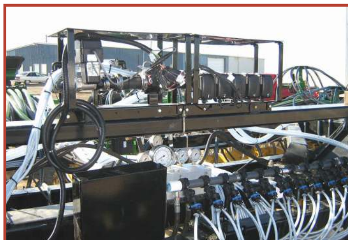
Auto Rate system with 5 sectional controls.
