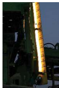
Tank Sight Gauge Light
